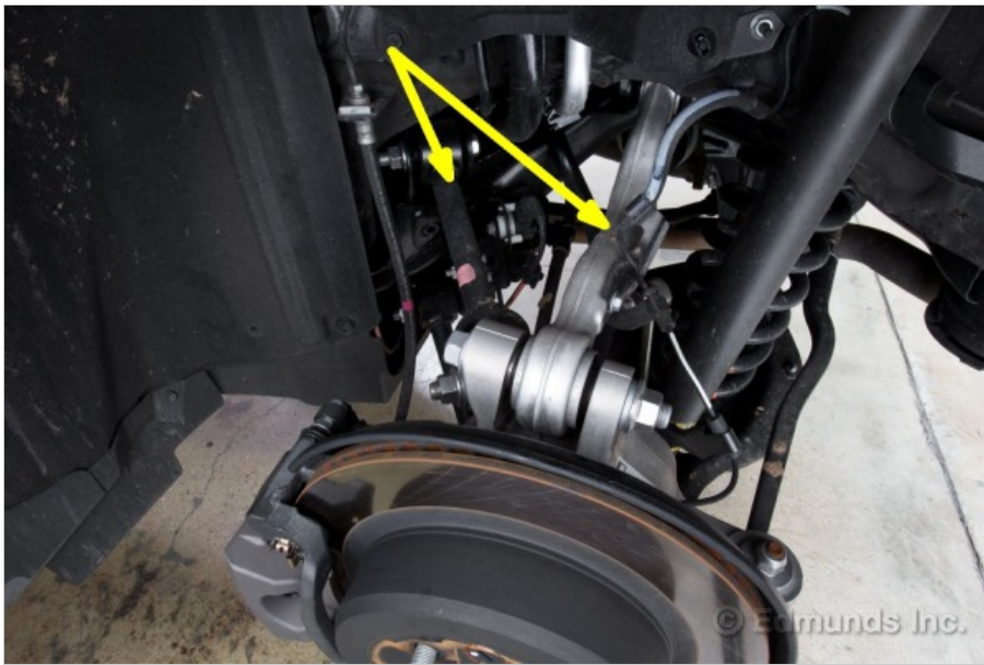
Like last year, the top end is located by a pair of upper links arrayed in the rough shape of an upper A-arm (green).
